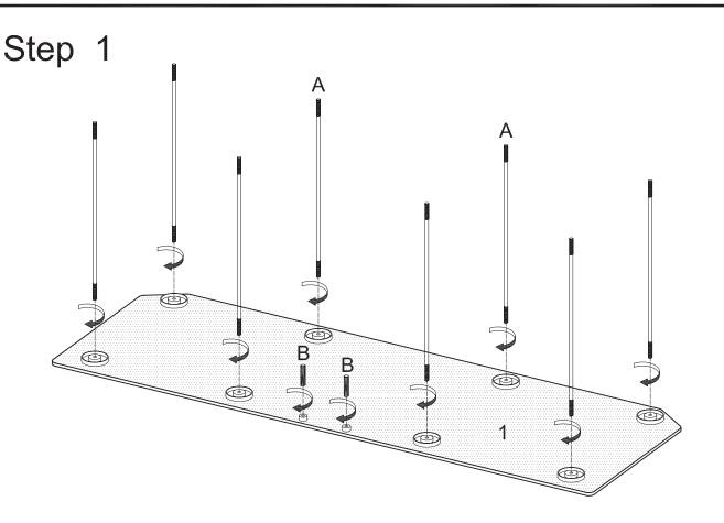
Carefully lay glass (1) upside down on a soft surface. Screw long rods (A) and short rods (B) into the appropriate metal plates of glass (1).
